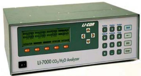
**Licor 7000:** Measurement of incubated soil respiration
